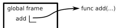
Figure 4: The result of evaluating " from operator import add" in the global frame.
